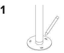
Place the Tool Kit in the desired location. Use a marker or pencil to outline the holes of the flange onto the base material.
