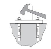
Thread nuts onto anchors, leaving approximately 1/4" of the anchor protruding, and tap into surface. Tighten nuts down to secure the stand.
