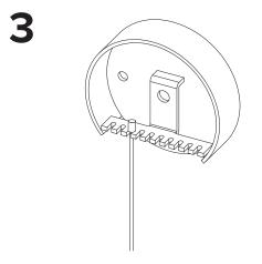
Once the base is installed, place the tool cables in the slots, and fasten the cap with the provided 3/8" tamper-resistant bolt.
