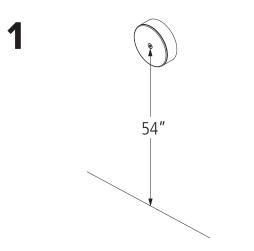
The Tool Kit wall-mount should be installed with the center of the Tool Kit 54" above the ground.
