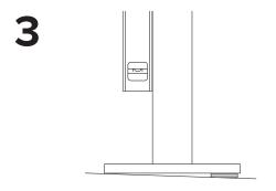
Place Tool Kit (and washers to level rack if necessary) over holes.
